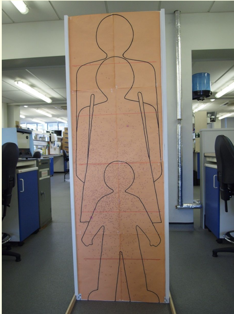
Typical results using the acid-indicator method for the jet air dryer
